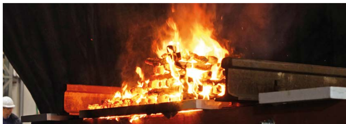
Fig.1: Fire test on open steel beam construction (here: Fire on the upper surface of the bridge track)
