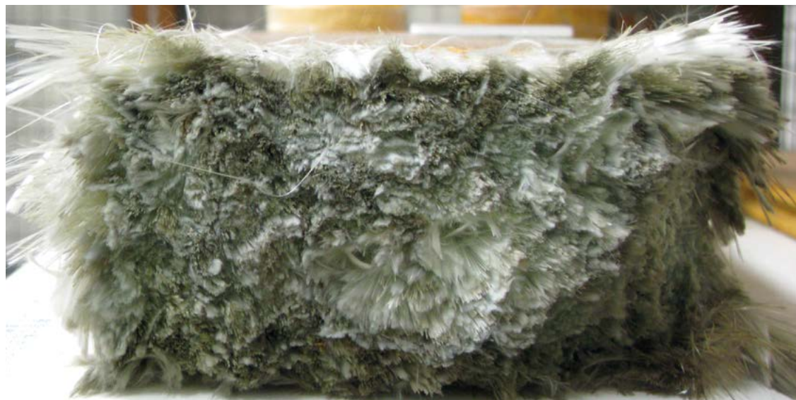
Fig. 1: Cross section of FFU synthetic sleeper showing amount of glass fibres
